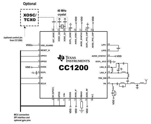
Figure 6-1. Typical Application Circuit
