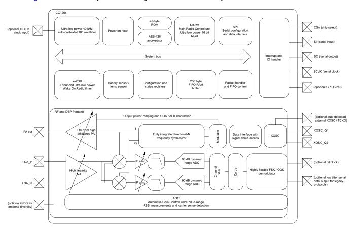
Figure 5-1. System Block Diagram
