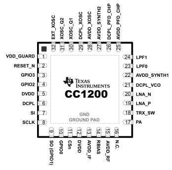
Figure 3-1. Package 5-mm × 5-mm QFN
