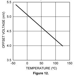
Current Sense Amplifier Input Offset Voltage vs Temperature 175
