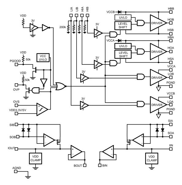
Figure 2. Block Diagram
