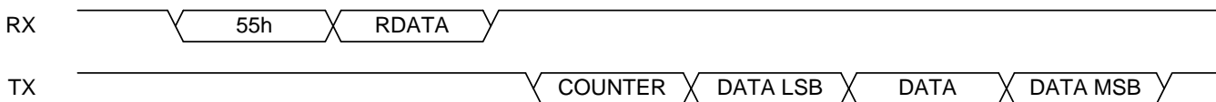
Figure 64. Manual Data Read Mode Using the Conversion Data Counter (Continuous Conversion Mode)
