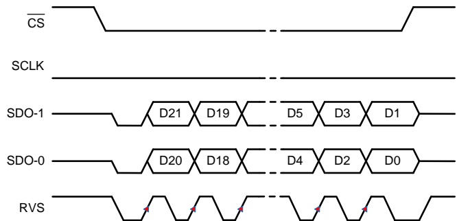
Figure 75. SRC-INT-DS: SRC, INTCLK, Dual SDO, SDR
