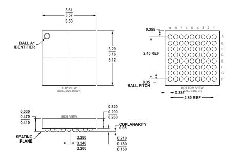
Figure 20. 72-Ball Wafer Level Chip Scale Package (WLCSP) (CB-72-3) Dimensions shown in mm
