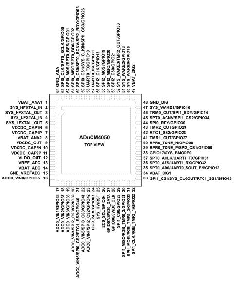
Figure 19. 64-Lead LFCSP Configuration
