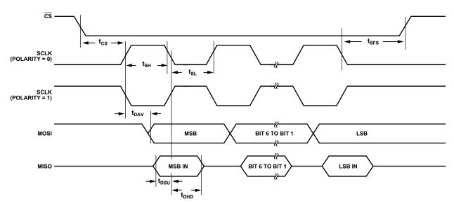
Figure 8. SPI Master Mode Timing (Phase Mode = 1)
