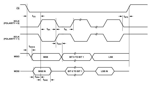
Figure 11. SPI Slave Mode Timing (Phase Mode = 0)
