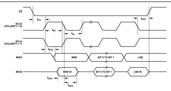
Figure 10. SPI Slave Mode Timing (Phase Mode = 1)
