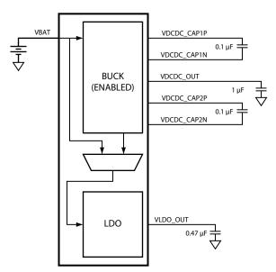
Note: For designs in which the optional buck is not used, the following pins must be left unconnected—VDCDC\_CAP1P, VDCDC\_CAP1N, VDCDC\_OUT, VDCDC\_CAP2P, and VDCDC\_CAP2N.
