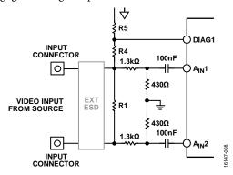
Figure 8. Diagnostic Connections
