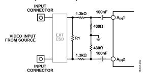
Figure 7. Differential Input Network
