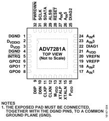
Figure 4. Pin Configuration
