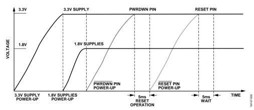
Figure 5. Optimal Power-Up Sequence
