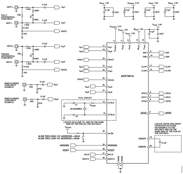
Figure 14. Typical Connection Diagram
