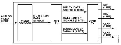
Figure 9. MIPI Tx Output Stage of the ADV7281A
