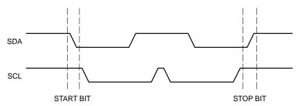
Figure 3. Start/Stop Timing
