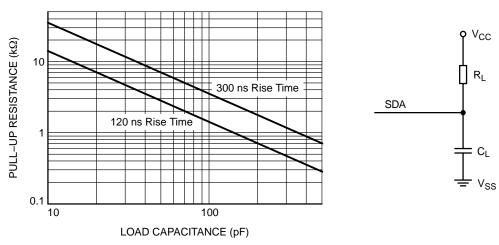
Figure 2. Pull-up Resistance vs. Load Capacitance
