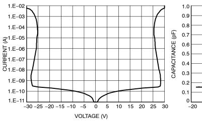
Figure 9. Typical IV Characteristics
