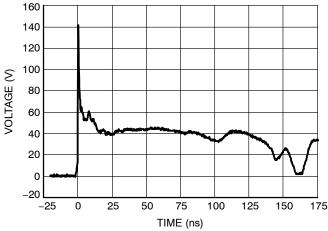
Figure 1. Typical IEC61000-4-2 + 8 kV Contact ESD Clamping Voltage
