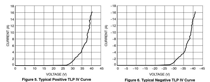
NOTE: TLP parameter:  $Z_0 = 50 \Omega$ ,  $t_p = 100 \text{ ns}$ ,  $t_r = 300 \text{ ps}$ , averaging window:  $t_1 = 30 \text{ ns}$  to  $t_2 = 60 \text{ ns}$ .
