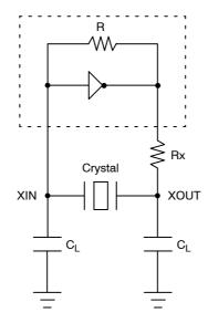
$$\label{eq:CL} \begin{split} &C_L=2^{\star}(C_P-C_S),\\ &Where \ C_P=Load\ capacitance\ of\ crystal\ from\ crystal\ vendor\ datasheet.\\ &CS\ =\ Stray\ capacitance\ due\ to\ CIN,\ PCB,\ Trace,\ etc. \end{split}$$
