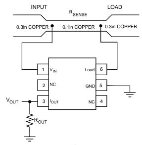
Figure 14. Using PCB Trace for RSENSE
