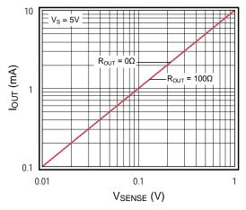
Figure 4. V<sub>SENSE</sub> vs. Output Current
