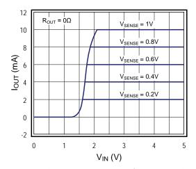
Figure 8. Transfer Characteristics
