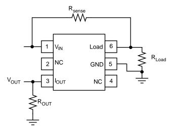
Figure 2. Typical Circuit
