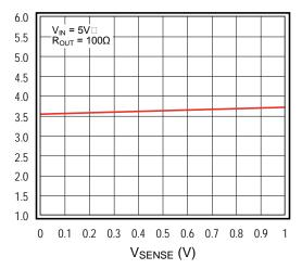
Figure 12. Supply Current vs. V<sub>SENSE</sub>
