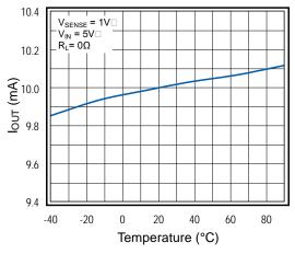
Figure 6. Output Current vs. Temperature
