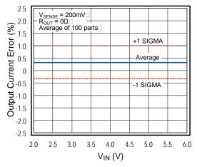
Figure 11. V<sub>IN</sub> vs. Output Current Error
