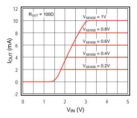
Figure 9. Transfer Characteristics
