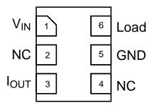
Figure 3. Pin Assignment (Top Through View)
