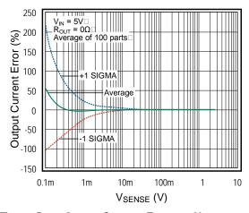
Figure 5. Output Current Error vs. V<sub>SENSE</sub>
