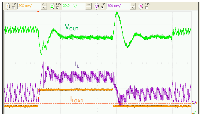
图22. 负载瞬态, 150 mA 至400 mA, V_{IN}=3.6V , t_{RISE}=t_{FALL}=100 ns, 5 \mu s /div.
