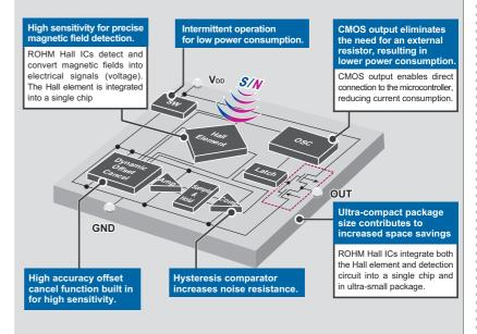
Block diagram is about omnipolar detection hall IC and unipolar detection hall IC series.
