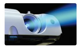
High-efficacy LEDs enable long operating life in portable projectors. Common-anode connected RGB LEDs are used to reduce wiring and ensure low thermal impedances for the LED. This requires the use of four high-efficiency, low-voltage LED drivers.
