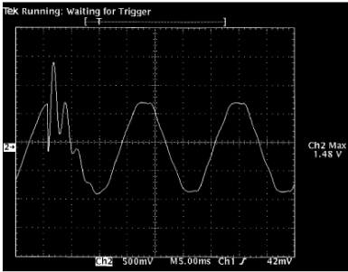
TYPICAL LOW FREQUENCY DECAYING RINGWAVE
