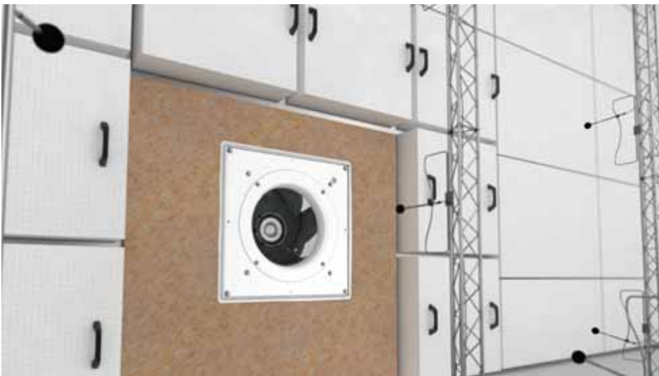
Fig. 1a: Centrifugal fan set up on test stand with free inlet, noise measurement microphones on suction side
