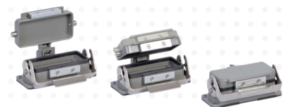
When the spring closes the cover, magnets tightly squeeze the cover closed. The result is an automatic IP66 seal that reaches a full IP69 seal when the lever is locked
