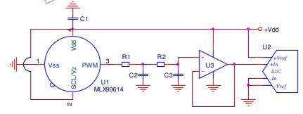
With R1=47k, R2=470k, C2=C2=1uF, the ripple (again at 5V, 50%, 1kHz) seen by the ADC will be less than 20 uV. Note that this ripple reduction comes with significantly increased settling time (3 seconds for this case). Certainly, a cost-effective approach might be to use a first order RC network between the MLX9614 and the ADC in conjunction with digital filtering of the ADC output.
