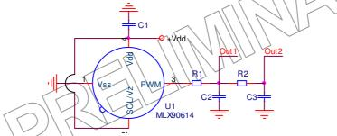
If this amount of ripple is unacceptable, a more complicated schematic could be used, like
