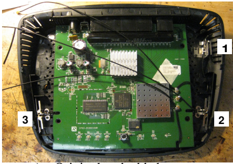
a) Original embedded antennas (referred as Baseline)
