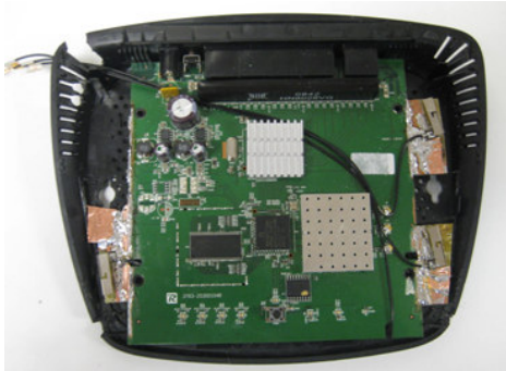
b) WLAN Prestta antennas on the real board
