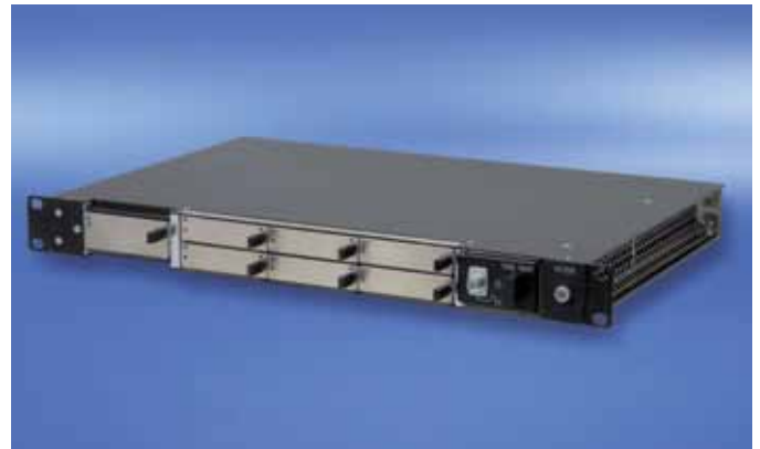
MicroTCA system: 1 U for 6 single mid-size AMC modules: larger air inlet and exit surfaces are obtained through specially shaped side panels.
