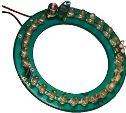
infrared light tuned to a specific wavelength, they are inherently directional, and they have significantly lower power consumption than other light sources. By mounting the LEDs to a ring-shaped PCB substrate designed to fit the diameter of a standard camera lens, the LED assembly is always aimed in the same direction as the lens to provide optimal infrared illumination.
