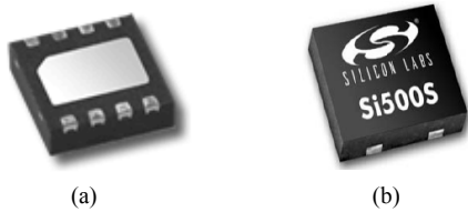
Fig. 19 (a) Mobius Microsystems’ 3x3mm 2 CHO [37] and (b) Silabs’ 4x3.2mm 2 Si500S Silicon Oscillators [38]
