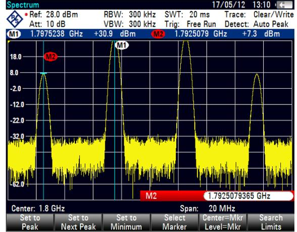
Figure 9: Two tone test measurement when  $P_{IN} = 25$  dBm
