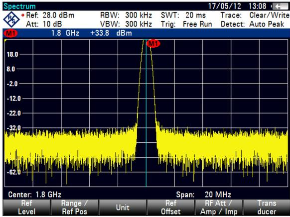
Figure 7: The measured output signal when  $P_{IN} = 24$  dBm
