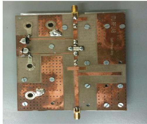
Figure 5: The fabricated circuit
