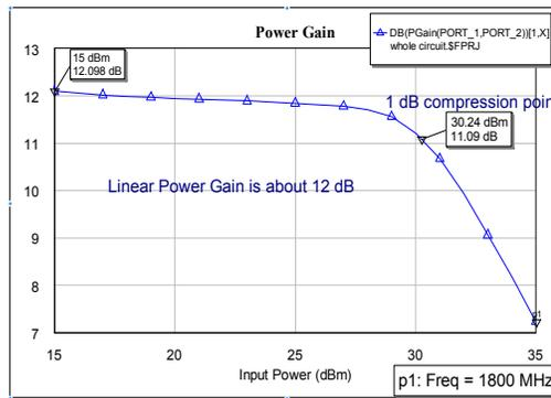
Figure 1: The power gain of the circuit
