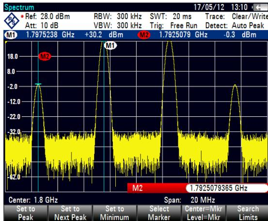
Figure 8: Two tone test measurement when  $P_{IN} = 24$  dBm
