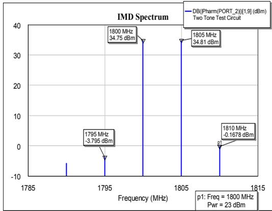
Figure 3: Intermodulation Spectrum ( $P_{IN}=23$  dBm)
