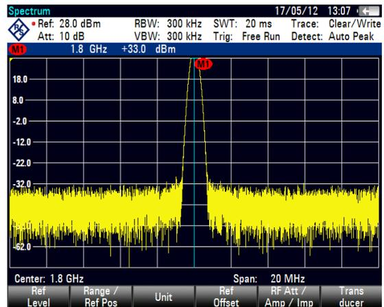
Figure 6: The measured output signal when  $P_{IN} = 23$  dBm
