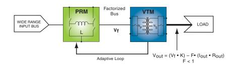
Under **remote loop control**, illustrated in Fig. 9, the voltage at the load is sensed and fed back to the PRM. This feedback protocol provides the most accurate load regulation – within +/- 0.2% – but may require isolation in the feedback path.
