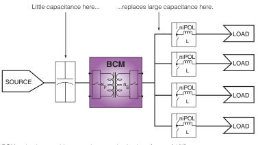
BCM technology enables capacitance reduction by a factor of 1/K<sup>2</sup> by locating at the input of the BCM instead of output (load).
