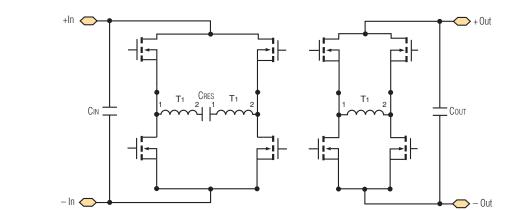
Figure 2 – Simplified schematic of the Sine Amplitude Converter
