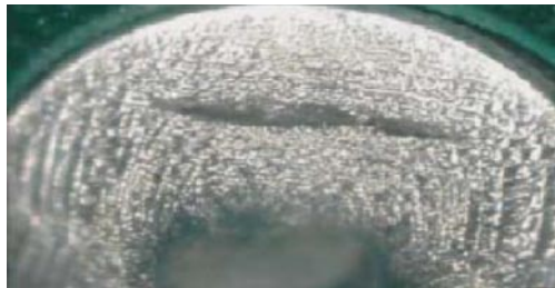
Figure 11 Shrink hole/Hot tear
