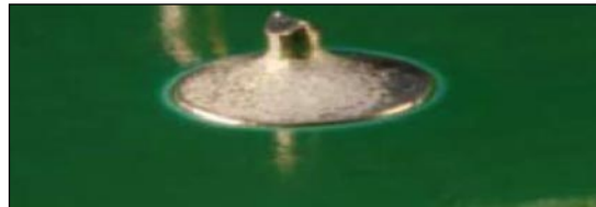
Figure 3 Example of acceptable protrusion of soldered lead.
