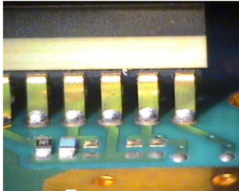
Figure 7 Good joints on board top side
