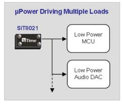
portable audio designWhen a MEMS-based  $\mu$ Power oscillator replaces a quartz oscillator, the power savings are even more dramatic. In a portable audio application for example, a SiT8021 oscillator operating at 3.072 MHz draws only 60  $\mu$ A compared to a quartz oscillator at 2.5 mA. In this case, the power consumption is 98% lower. This can effectively extend battery life by a full day – a huge improvement.
