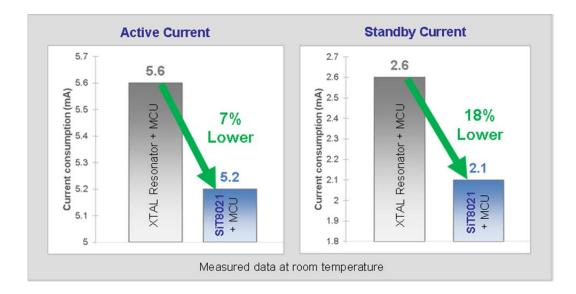
In addition to consuming less system power, SiTime's µPower oscillators – measuring only 1.5 x 0.8 mm – consume less board space, an important factor since many power sensitive products are also space sensitive. (See related blog: Shattering the Limits of Power, Size and Weight)
