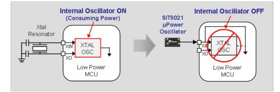
When a µPower oscillator replaces a crystal XTAL, the combined current consumption of the oscillator + MCU is lowered by 7% during the active state. Whereas in standby mode, 18% savings can be realized. During standby, the oscillator consumes only  $\leq$  0.9 µA because all internal circuits are turned off with the exception of the MEMS oscillator circuit and the ST pin detection logic.
