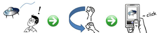
Figure 6. Gesture recognition UI: quickly turn on camera by hand waving the character "C".
