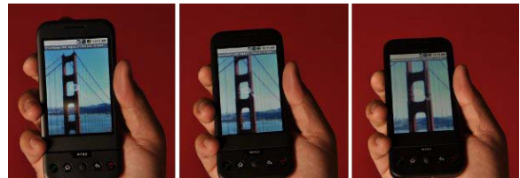
Figure 2. Gesture recognition UI. User can zoom in the picture by simply tilting the phone.
