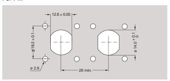
**Note:** PY• is also designed for snap-on fixing into customer housing. Consult factory for information. – Socket mounting nut torque = 1.5 Nm.
