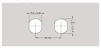
Note: socket mounting nut torque = 0.8 Nm.
