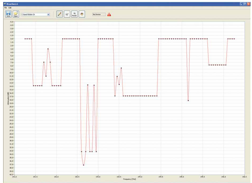
Screenshot of WaveSketch application showing user-defined filter shape created by the WaveSketch drag and drop interface
