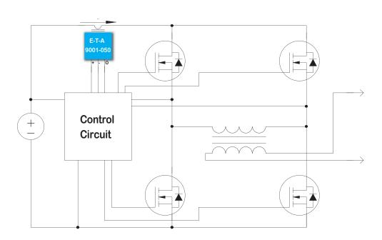
This application is similar to the three phase inverter. In this case, the detector is shown in the positive bus to the bridge, although it could have been just as easily placed in the ground bus. It makes no difference from a circuit perspective. However, from a packaging perspective, it provides some flexibility. This flexibility in placement can prove to be an advantage during the printed circuit board layout phase of the design.
