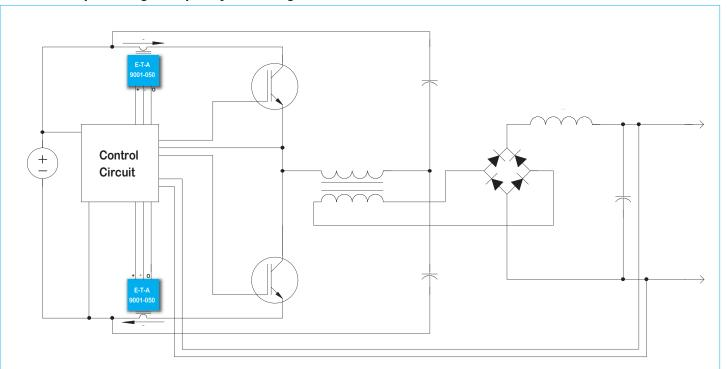
In this schematic of a high frequency half bridge IGBT based converter, two detectors are used to provide protection against over currents due to a variety of conditions. These include: shoot through, transformer saturation, output overload and transient output conditions.
