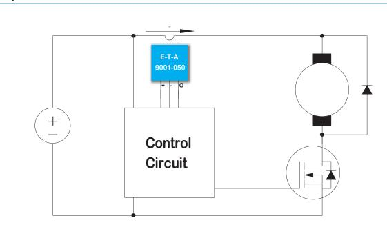
In this case, the detector can be located in the positive bus, between the negative side of the motor and the FET, or in the negative bus. All three locations provide equivalent protection. Similar to Example 2, the placement of the detector may be dictated by space considerations during the printed circuit board layout phase of the design.
