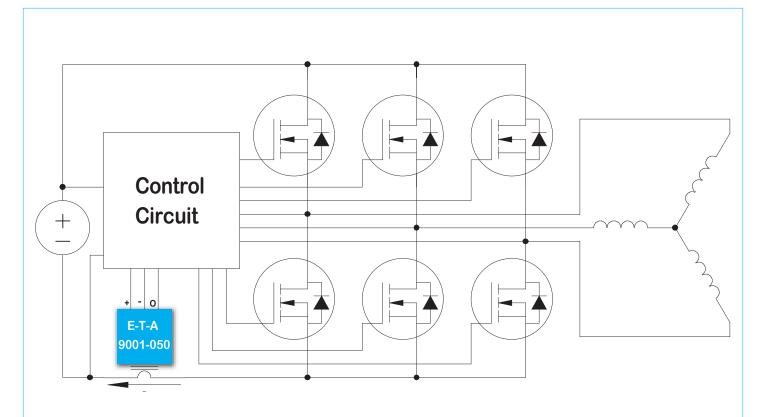
In this circuit, current must be sensed in the bridge to protect the power transistors against over current conditions. The over current conditions can be caused by transient loads on the output of the inverter, or shoot through conditions caused by noise in the control circuitry or intermittent logic problems.
