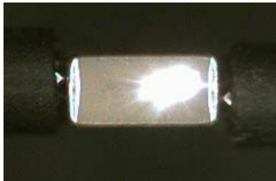
Figure 8. Side view of voltage breakdown of HVArc Guard™ 1812 case size X7R 150nF MLCC
