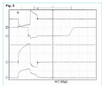
contributes a measurement error to trace R2. Although a low inductance shunt is used, it does have 10 nH of inductance which adds a voltage drop not representative of the current value. In this case, this inductance provides a 1 volt drop at a current rise rate of 100 A/ $\mu$ s. This can be seen at the turn on of the MOSFET where the voltage across the shunt instantaneously jumps to 1 volt, and during the turn off phase when the voltage instantaneously goes negative.
