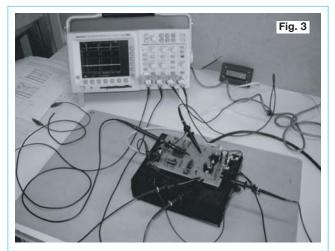
As described in the protection scheme, the logic section of the circuit consists of a microcontroller driving the clock input of a D flip flop with the output of the flip flop driving a gate MOSFET gate driver. The output of the OCD is fed back to clear the flip flop which turns the MOSFET gate drive off when an over current event is detected. Figure 3 displays the test set up.
