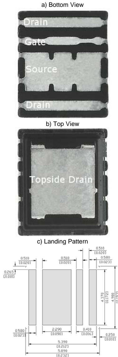
Figure 2. Photograph of the new PolarPAK MOSFET, with landing pattern
