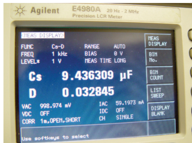
Figure 4. Capacitance measurement of 10 \mu F capacitor using ALC function.
