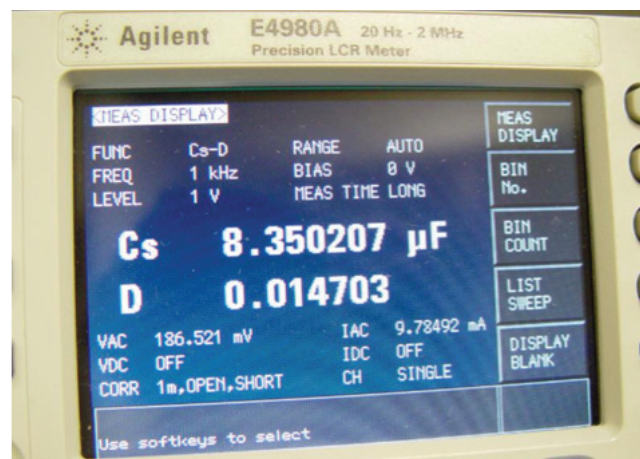
Figure 3. Capacitance measurement of 10 \mu F capacitor.
