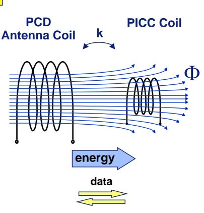
PCD: Proximity Coupling Device ("Reader") PICC: Proximity Chip Card ("Card")
