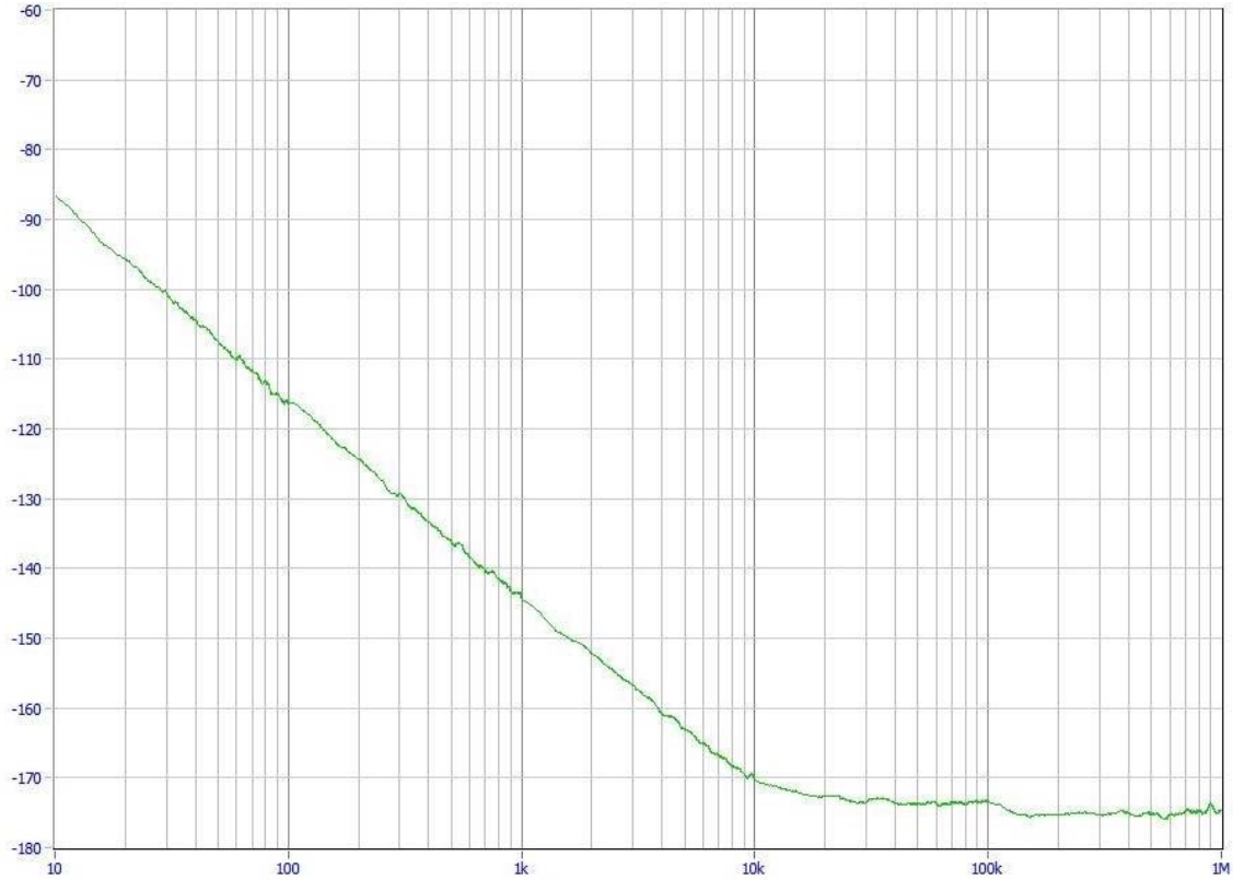
Typical Phase Noise at 100 MHz
