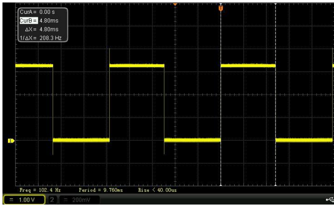
Figure 11. Maximum pulse width at 100Hz output frequency
