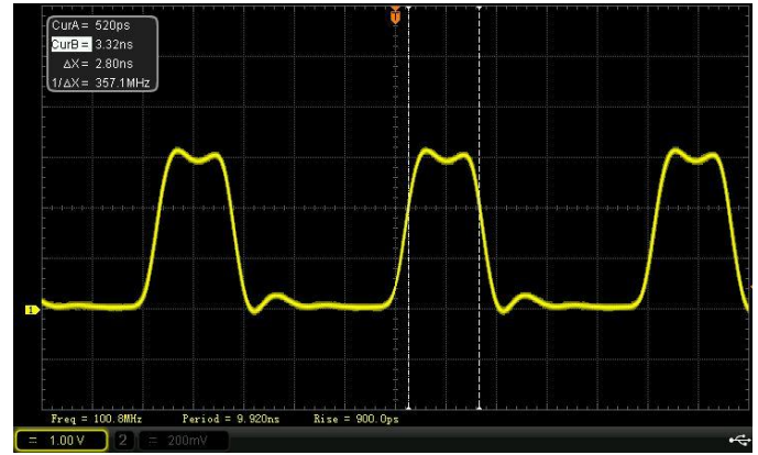
Figure 20. 2.8ns pulse width at 100MHz
