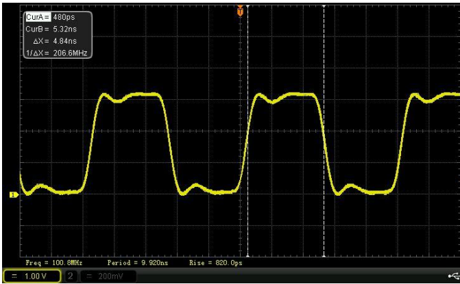
Figure 18. 4.84ns pulse width at 100MHz
