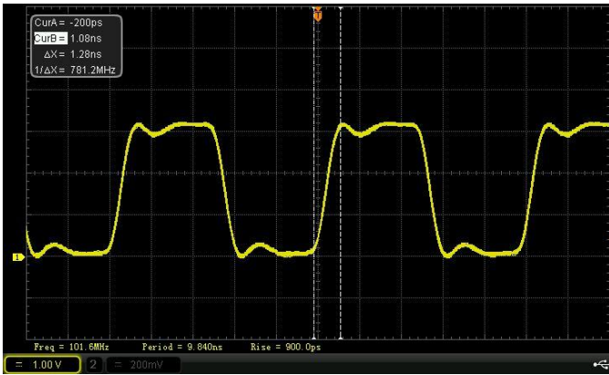
Figure 19. 1.28ns rise time at 100MHz
