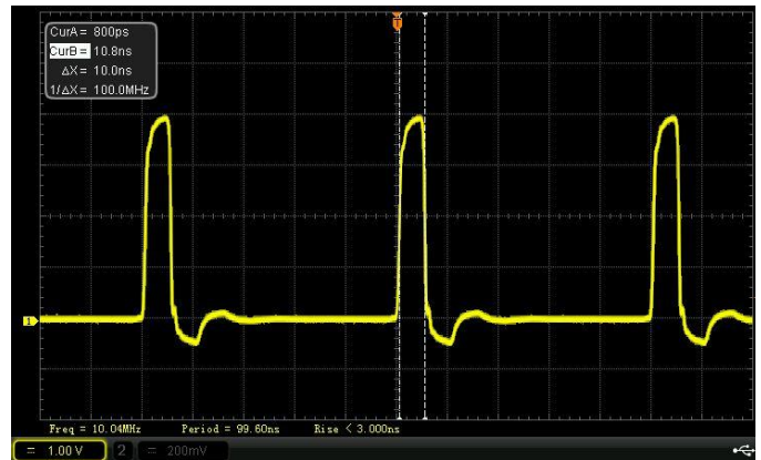
Figure 15. 10ns pulse width at 10MHz output frequency
