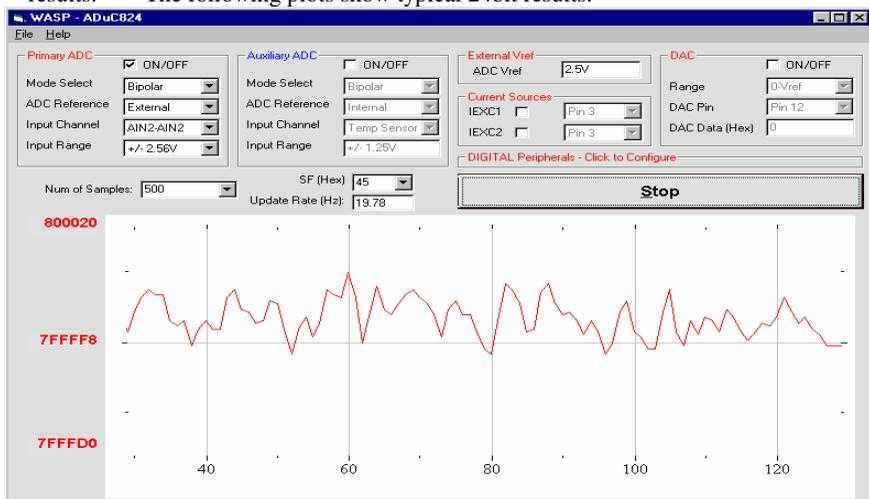
11. When all the samples are collected the WASP immediately launches the Analysis window. This window displays some mathematical analysis on the ADC conversions, including RMS noise (in  $\mu\text{V}$  and bits) and Peak-to-Peak Noise (Code Distribution,  $\mu\text{V}$  and Bits). The most important performance figures are highlighted in Red.
