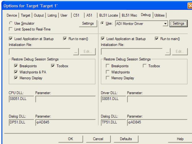
Click on Settings at the top right. Select 1-Pin Pod and the COM port assigned to the emulator as shown below. Use Device Manager to identify the appropriate COM port as describer previously.
