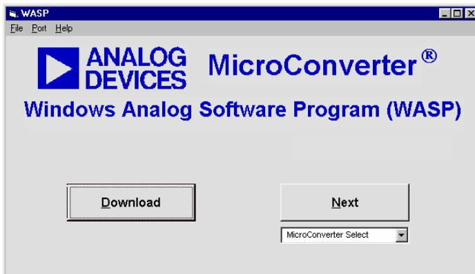
**Note:** The **NEXT** button bypasses the 'Download' sequence and can be used if the WASP code is already downloaded and running on the MicroConverter. To identify the MicroConverter for the WASP software the user should select the appropriate MicroConverter from the "MicroConverter Select" option box and then click on **NEXT**.
