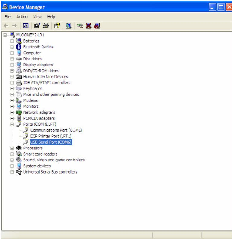
Note: The older versions of the Keil tools only work with COM port numbers of COM8 or lower. If your PC allocates a COM port number of COM9 or higher, then you will need to change the COM port to a lower number.
