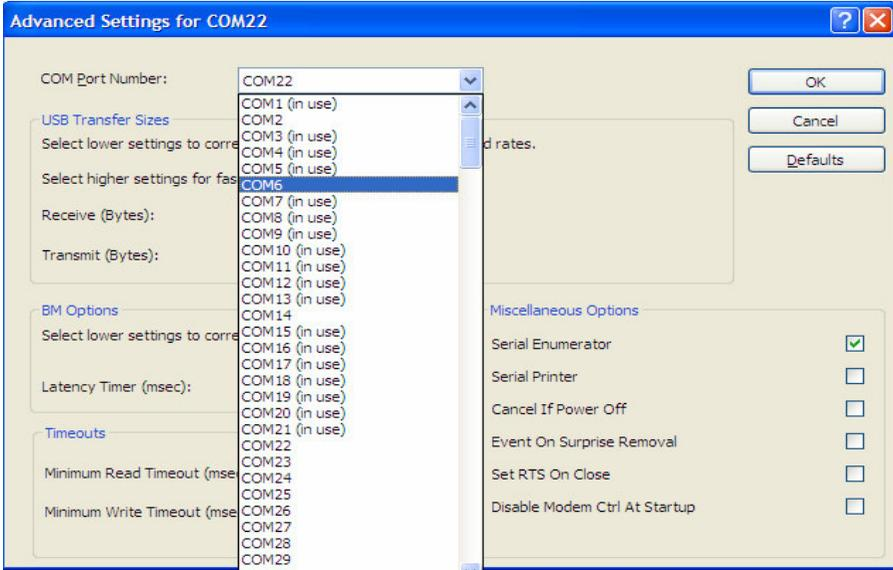
Click “OK” and return to the main Device Manager window. To update the newly selected COM port, unplug and re-plug the USB cable to the USB-EA dongle and the newly selected COM port should appear in the Device Manager window:
