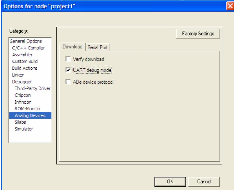
In the “Serial Port” menu, ensure the correct COM port is selected. As described earlier, use Device Manager to identify the correct COM port.
