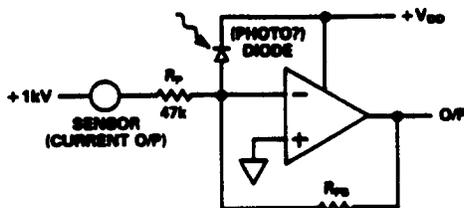
THE DIODE PROTECTS THE OP AMP UNDER FAULT CONDITIONS BY DIVERTING FAULT CURRENT (LIMITED BY  $R_p$ ) TO THE SUPPLY RAIL. THE DIODE SHOULD NOT BE PHOTO-RESPONSIVE. OTHERWISE FLUORESCENT LIGHTING MAY MODULATE ITS LEAKAGE CURRENT AT 100/120Hz AND CAUSE HUM. USE A PLASTIC DIODE - NOT A GLASS ONE.
