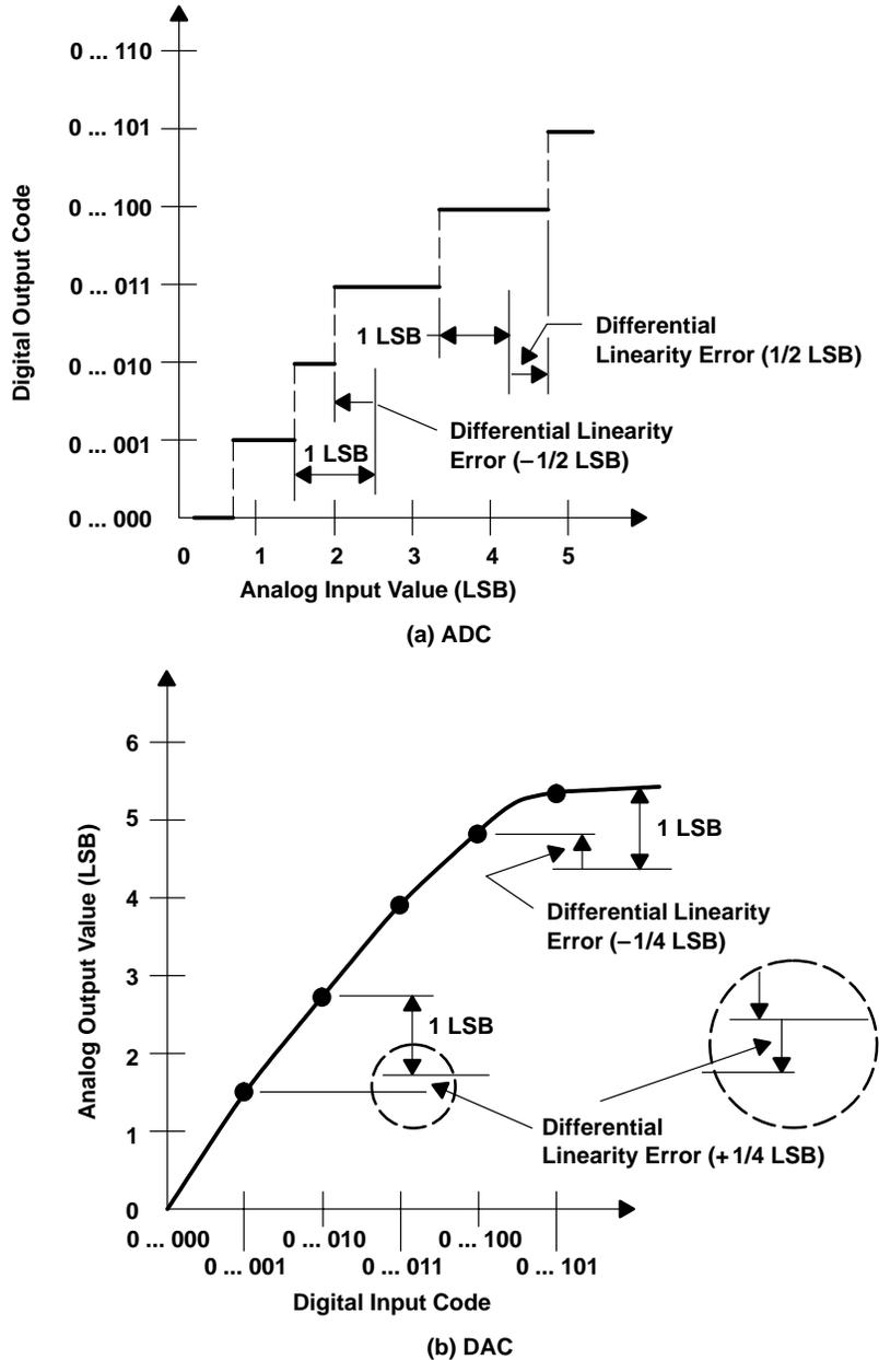
Differential Linearity Error of a Linear ADC or DAC
