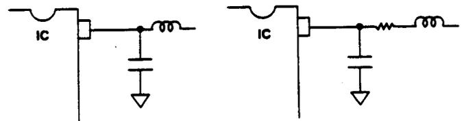
EQUIVALENT CIRCUIT OF DECOUPLED POWER LINE - RESONANT AT
