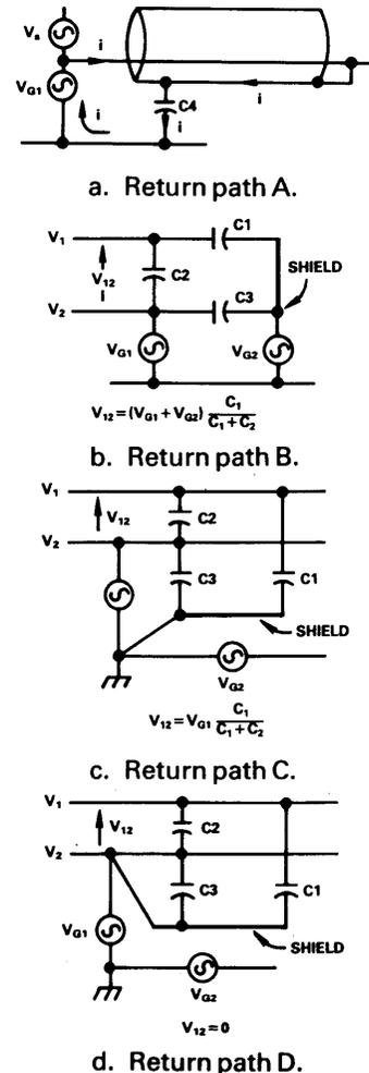
Figure 13. Equivalent circuits.
