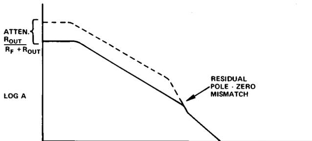
Figure 3c. Response of circuit 3a with finite  $R_{OUT}$ .
