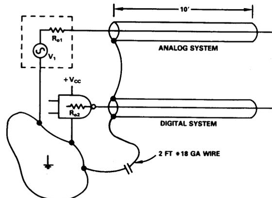
Figure 9. A situation that generates transient shield voltages.
