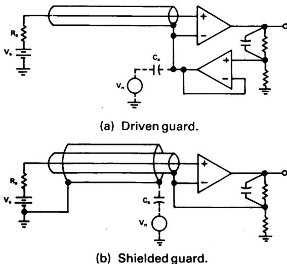
Figure 23. Avoiding noise pickup on the guard.
