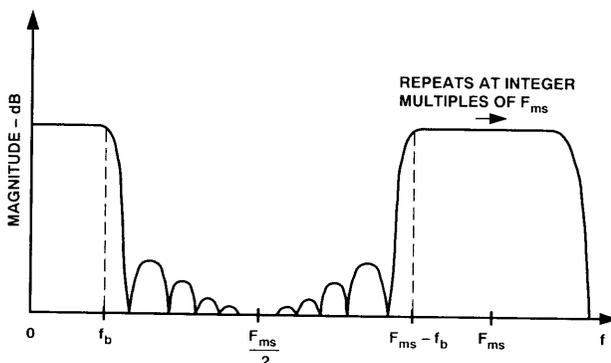
Thus it is the input noise energy in these bands  $[kF_{ms} \pm f_b]$  that must be removed by the antialiasing filter before the input signal is sampled by the converter.
