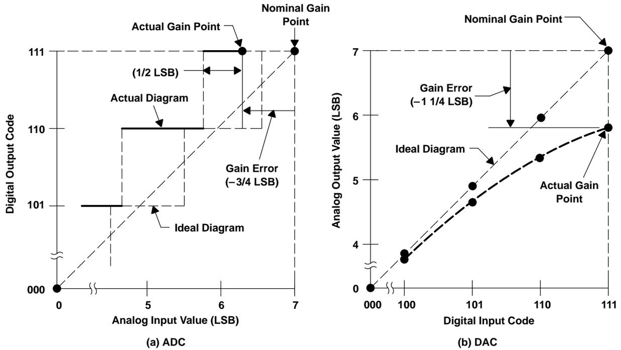
Gain Error of a Linear 3-Bit Natural Binary Code Converter
