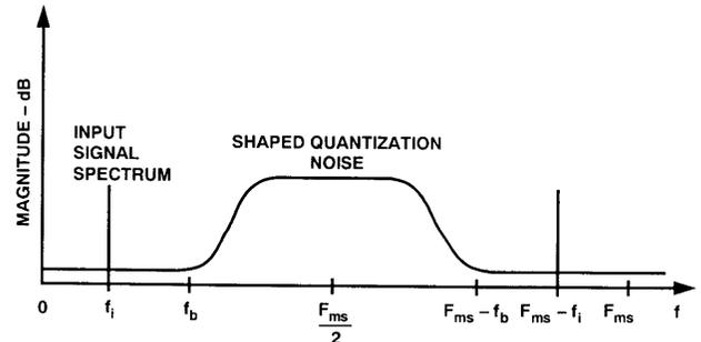
As shown, the spectral "sticks" (single frequencies) at  $f_i$  and  $F_{ms} - f_i$  correspond to an input signal, while the shaded area shows how the quantization noise has been pushed (shaped) beyond the bandwidth of interest,  $f_b$ .
