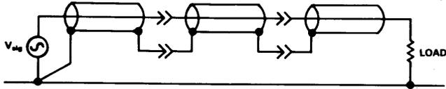
Figure 5. Shields must be interconnected if interrupted.
