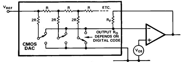
Figure 6. Variable output resistance of inverted R-2R ladder in CMOS and voltage-switching DAC's.
