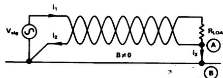
b. Incorrect connection forming ground loop.
