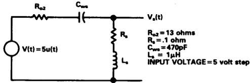
Figure 10. Equivalent circuit for generating shield voltage.
