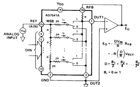
**a.** CMOS DAC connected for current steering. Input impedance is constant.
