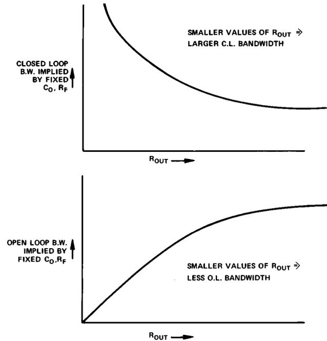
Figure 4. Effect of varying  $R_{OUT}$  ( $R_O'$ ) on open-loop and closed-loop bandwidth.
