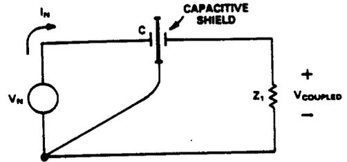
EQUIVALENT CIRCUIT ILLUSTRATES HOW A CAPACITIVE SHIELD CAUSES THE NOISE CURRENTS TO RETURN TO THEIR SOURCE WITHOUT FLOWING THROUGH Z1
