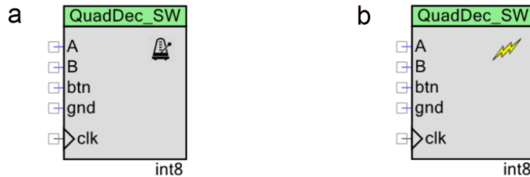
Figure 2. Component appearance in polling and interrupt modes: (a)-polling mode, timer clock appears on the symbol; (b)-interrupt mode, interrupt symbol appears on the symbol.
