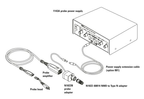
Figure 3. A complete InfiniiMax general-purpose probing system
