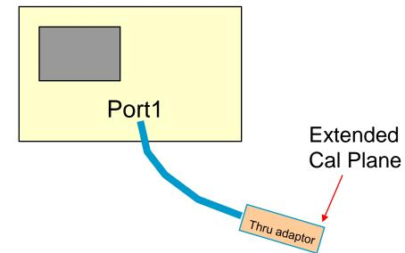
The estimated delay time of the unknown thru is acquired using the automatic port extension function.
