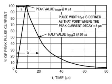
Figure 1. 8 x 20 μs Pulse Waveform
