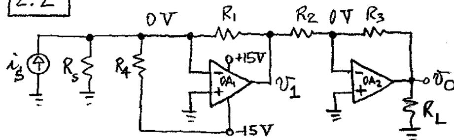
$$V_o = -\frac{R_3}{R_2} V_1 = -\frac{R_3}{R_2} \left[ -R_1 i_s - \frac{R_1}{R_4} (-15 \text{ V}) \right].$$
