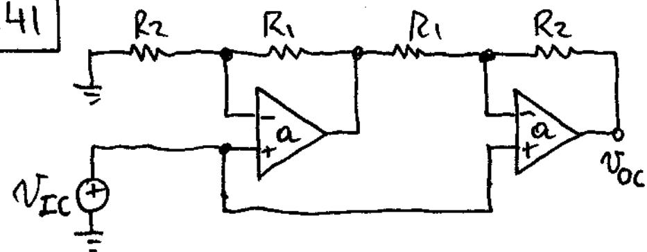
$$A = 1 + R_2/R_1 \Rightarrow R_2/R_1 = A - 1, R_1/R_2 = 1/(A-1)$$
