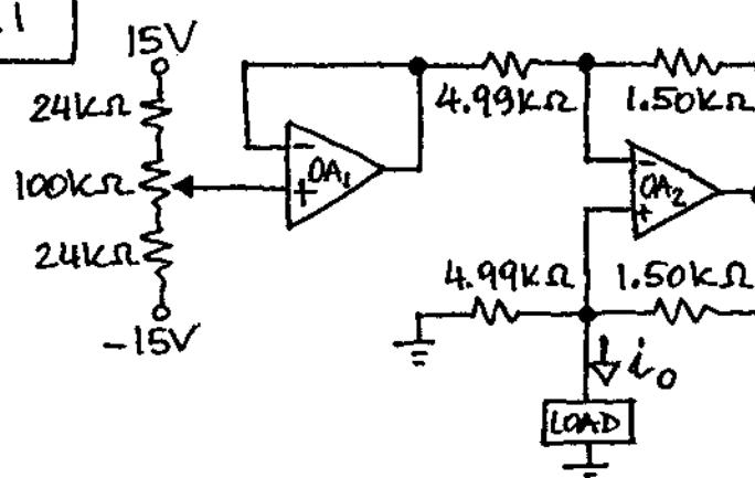
OA<sub>1</sub> provides a variable voltage from -10V to +10V, which OA<sub>2</sub> converts to a variable current from -2mA to +2mA.
