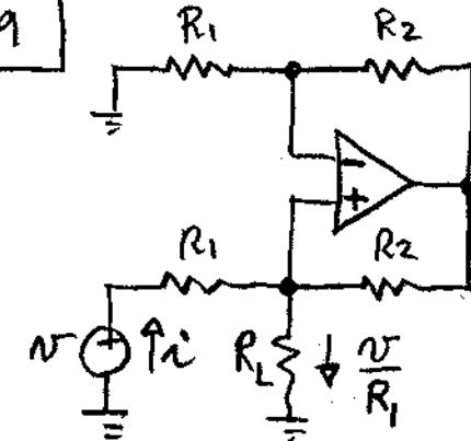
$$i = \frac{V - (V/R_1)R_L}{R_1}$$
