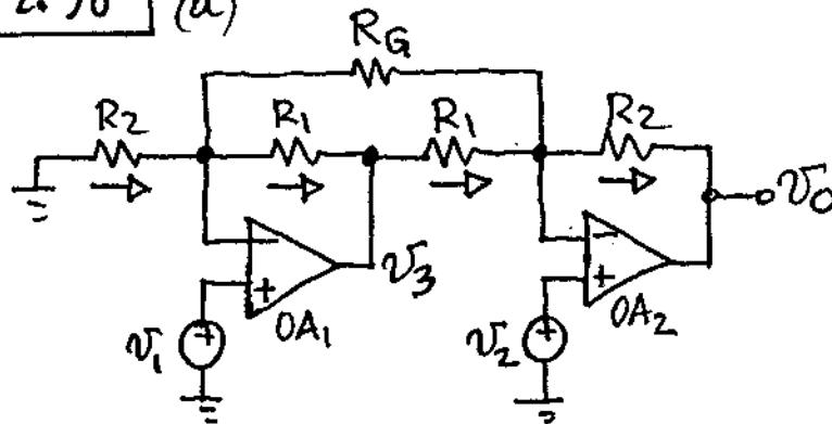
$V_{N1} = V_{P1} = V_1$ ,  $V_{N2} = V_{P2} = V_2$ . Applying KCL:
