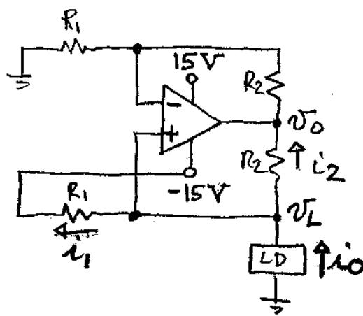
$R_1 = 15/1.5 = 10.0 \text{ k}\Omega, 1\% ; R_2 \leq 0.3 R_1$ . Use  $R_2 = 2.00 \text{ k}\Omega, 1\%$ . Then,  $V_0 = (1 + 2/10)V_L = 1.2V_L$ .
