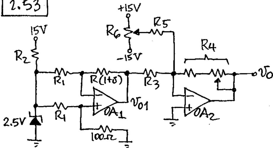
Let  $R_1 = 2.49\text{ k}\Omega$ . Then,  $\Delta T = 1^\circ\text{C} \Rightarrow \Delta V_{01} = [100/(100+2490)] \times 2.5 \times 0.00392 = 378.38\text{ }\mu\text{V}$ .
