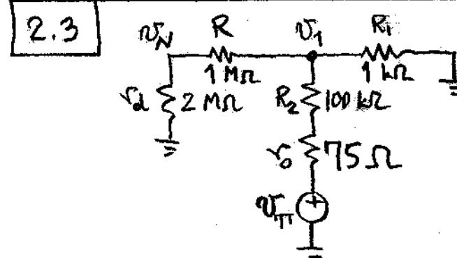
$$V_N = \frac{R}{R_a + R} V_1 = \frac{2}{3} V_1;$$
