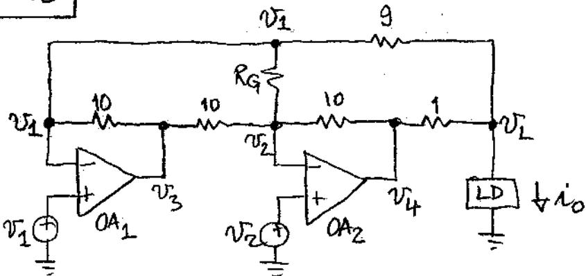
Summing currents at the inverting inputs of the op amps,
