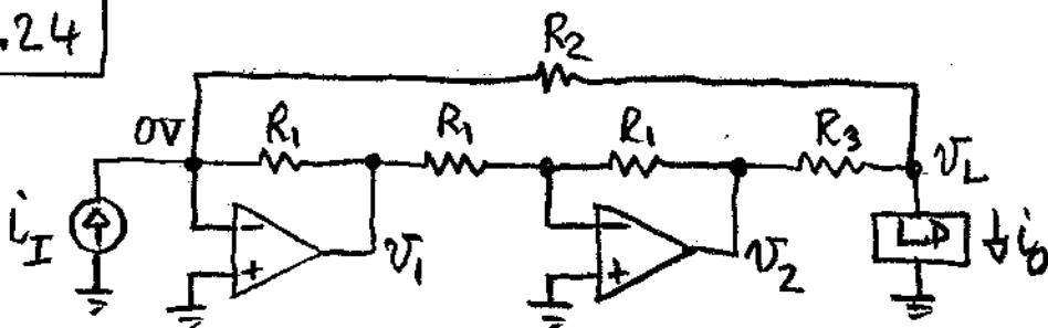
$$v_1 = -R_1 i_I - (R_1 / R_2) v_L; v_2 = -v_1 = R_1 i_I + \frac{R_1}{R_2} v_L.$$
