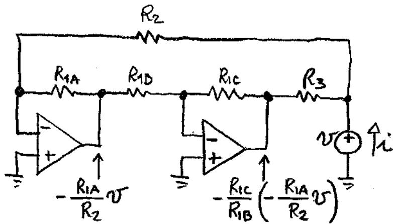
$$i = \frac{v}{R_2} + \frac{v - (R_{1A}R_{1B}/(R_2R_{1B}))v}{R_3}$$
