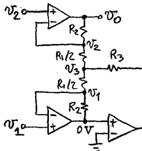
$$V_1 = \frac{R_2}{R_2 + R_1/2} V_3 \Rightarrow$$
