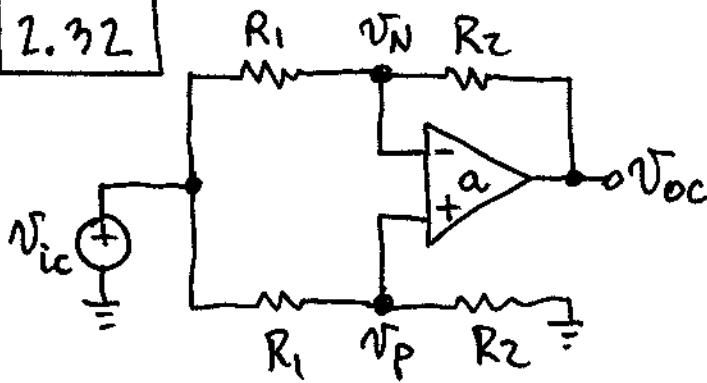
$$\begin{aligned} V_{oc} &= a(V_p - V_N) = a \left[ \frac{R_2}{R_1 + R_2} V_{ic} - \frac{R_2 V_{ic} + R_1 V_{oc}}{R_1 + R_2} \right] \\ &= a \left[ \cancel{\frac{R_2}{R_1 + R_2} V_{ic}} - \cancel{\frac{R_2}{R_1 + R_2} V_{ic}} - \frac{R_1}{R_1 + R_2} V_{oc} \right] \end{aligned}$$
