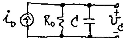
(a)  $i_0 = 1 \text{ mA}$ ;  $R_o = R_2 / (R_2/R_1 - R_4/R_3) = 4.42 / (4.42/15 - 3.978/15) = 150 \text{ k}\Omega$ ;  $R_o i_0 = 150 \times 1 = 150 \text{ V}$ ;  $\tau = R_o C = 150 \times 10^3 \times 10^{-7} = 15 \text{ ms}$ ;  $(1 + R_2/R_1)R_o i_0 = (1 + 3.980/15)150 \approx 190 \text{ V}$ .
