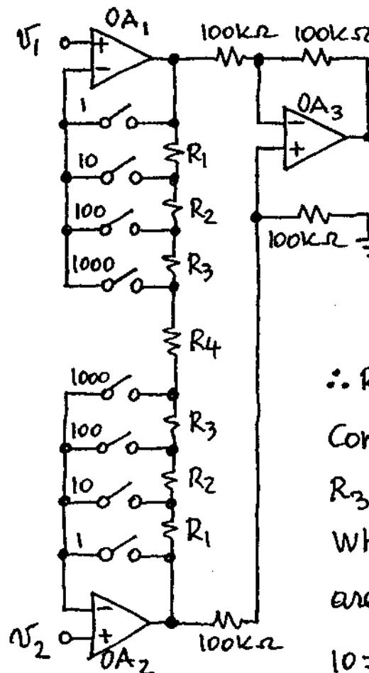
$$1000 = 1 + 2 \frac{R_1 + R_2 + R_3}{1}$$
