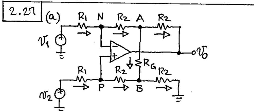
$$\text{KCL at } N: \frac{V_1 - V_N}{R_1} = \frac{V_N - V_A}{R_2}$$
