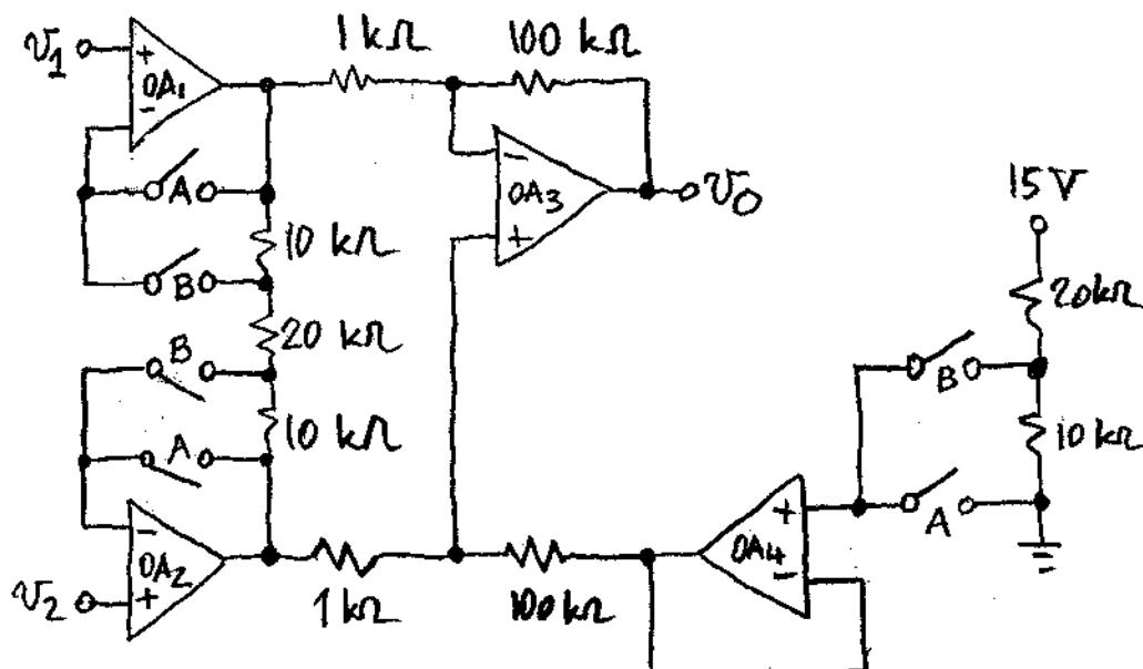
"A" switches closed  $\Rightarrow V_0 = 1 \times 100(V_2 - V_1) + 0 \text{ V}.$
