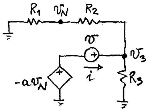
$$\begin{aligned}V_3 &= (1 + R_2/R_1)V_N = 1.99V_N; \quad -aV_N + V = V_3 \\ \Rightarrow V_N &= V/(1.99 + 10^3); \quad i = V_3/(R_1 + R_2) + \\ V_3/R_3 &= [1.99 \cdot V/(1.99 + 10^3)] / [(199 \parallel 1)10^3] \\ &= V/(500,995). \quad R_o = V/i \approx 501 \text{ k}\Omega.\end{aligned}$$
