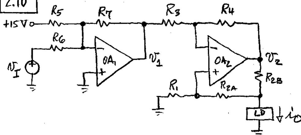
Let  $R_1 = R_3 = R_4 = 10\text{k}\Omega$ . Assume a maximum drop of 2 V across  $R_{2B}$ , so  $R_{2B} = 2/20 = 100\Omega$ . Then,  $R_{2A} = 10\text{k}\Omega - 100\Omega = 9.9\text{k}\Omega$ .
