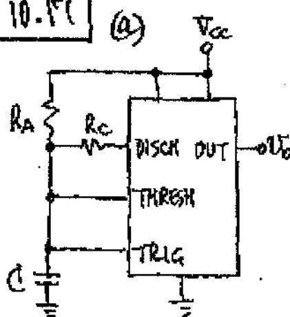
When Q inside the 555 is OFF, C charges toward  $V_{CC}$  via  $R_A$ , so  $T_H = R_A C \ln 2$ . When Q is saturated, C discharges toward  $V_{DD} = \frac{R_C}{R_A + R_C} V_{CC}$
