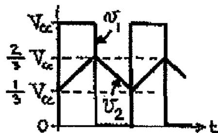
$V_1$  alternates between 0 and  $V_{cc}$ . To make  $i_C$  alternate between two symmetric values about zero, we must offset the integrator, as shown. Then,  $i_C = (V_1 - V_{cc}/2)/R = \pm V_{cc}/2R$ . We observe that as  $V_2$  alternates between  $(1/3)V_{cc}$  and  $(2/3)V_{cc}$ ,
