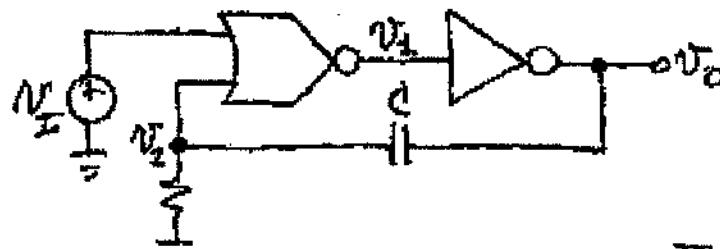
$$T = R C \ln \frac{0 - V_{DD}}{0 - V_T} = R C \ln \frac{1}{0.4}$$
