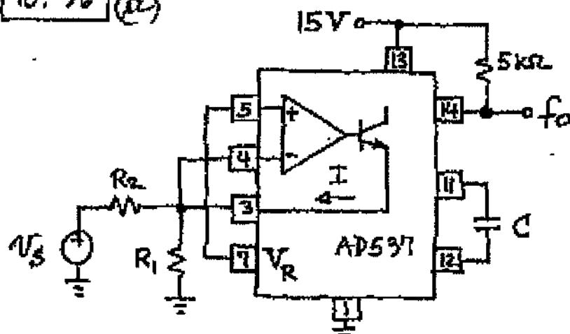
$V_N = V_P = V_R = 1.00 \text{ V}$ . With  $V_I = +10 \text{ V}$ , impose  $I = 0$ . This requires  $R_2 = 9 R_1$ . With  $V_I = -10 \text{ V}$ , impose  $I = 1 \text{ mA}$ . This requires  $1/V_2 + 1/R_1 = 1$ . Combining & solving,  $R_2 = 20.0 \text{ k}\Omega$ ,  $R_1 = 2.22 \text{ k}\Omega$ ;  $20 \times 10^3 = 10^{-3} / (10C) \Rightarrow C = 5 \text{ mF}$ .
