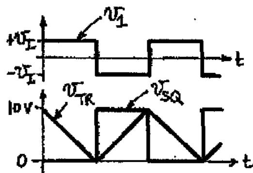
$$\begin{aligned} AV &= 10\text{V}, I = V_I/R, \\ \text{and } At &= T/2, \text{ we} \\ \text{get } T &= 20RC/V_I, \\ \text{or} \\ f_0 &= \frac{V_I}{20RC}. \end{aligned}$$
