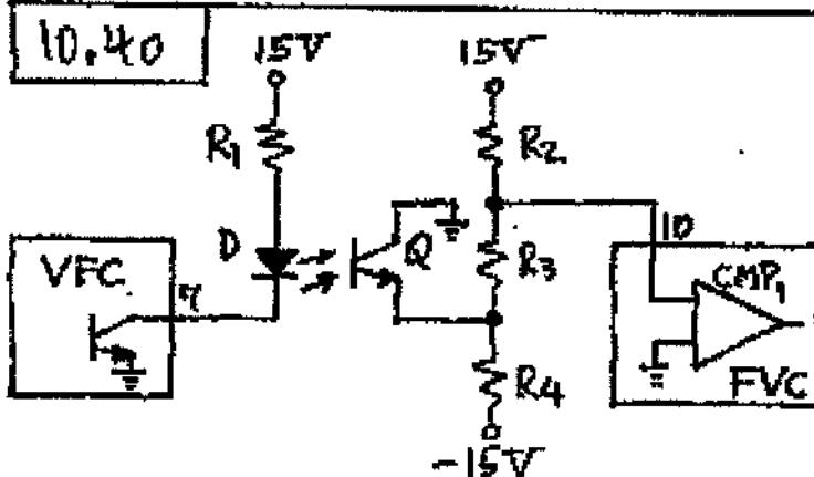
To ensure  $I_F \approx 10\text{ mA}$ , use  $R_1 = 1.3\text{ k}\Omega$ . Impose a  $\pm 3\text{ V}$  swing at pin 10 of the FVC. Then, when Q is off, we want
