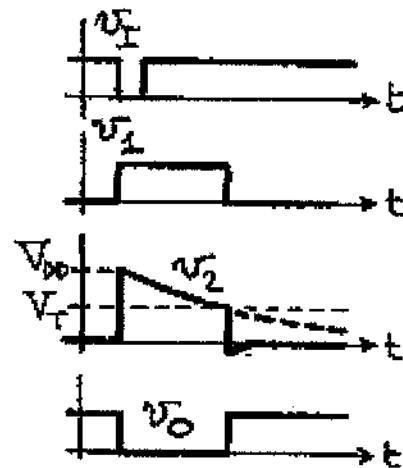
$V_1$  must be a negative-going pulse and  $R$  must be returned to ground to ensure a logic high at the upper input to  $G_1$ . Using  $V_0 = V_{DD}$ ,  $V_{DD} = 0$ ,  $V_1 = V_T$ , and  $\Delta t = T$  in Eq. (10.3) we obtain  $T = RC \ln(V_{DD}/V_T)$ .
