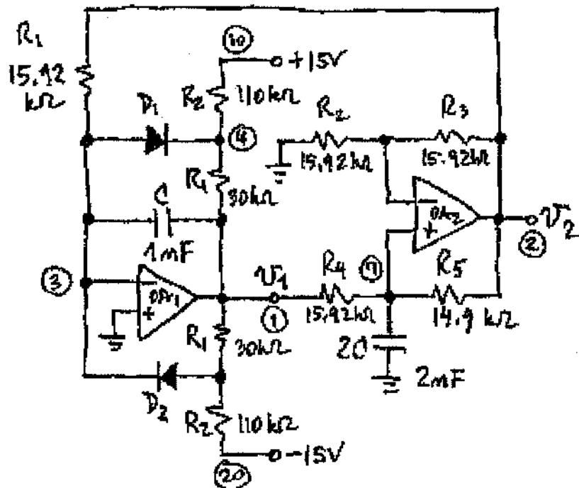
Running the accompanying PSpice program with two different sets of initial conditions gives the plots shown. Because of nonidealities, the actual frequency of oscillation is 9.74 kHz.
