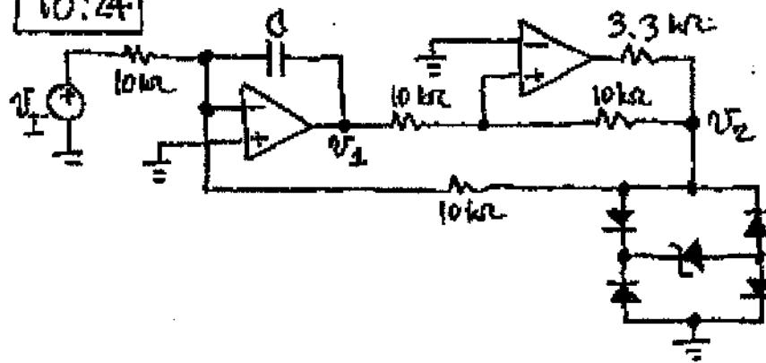
$V_2 = \pm (V_{25} + 2V_{D(on)}) = \pm 5V$ ;  $V_T = \pm 5V$ .
