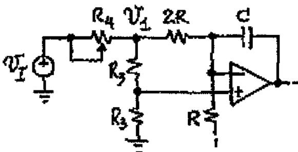
$$f_0 = \left(1.25 \frac{\text{kHz}}{V}\right) V_1$$
