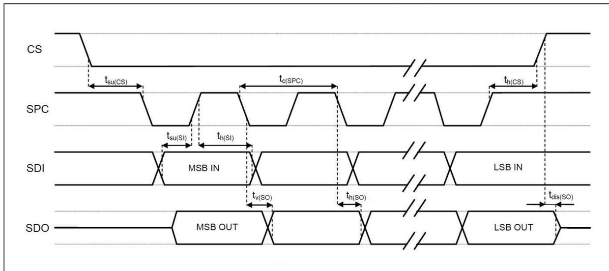
Note: Measurement points are done at  $0.2 \cdot V_{dd\_IO}$  and  $0.8 \cdot V_{dd\_IO}$ , for both input and output ports.
