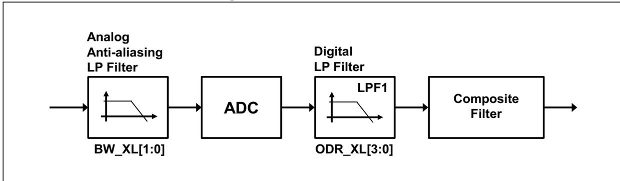
Figure 5. Accelerometer composite filter
