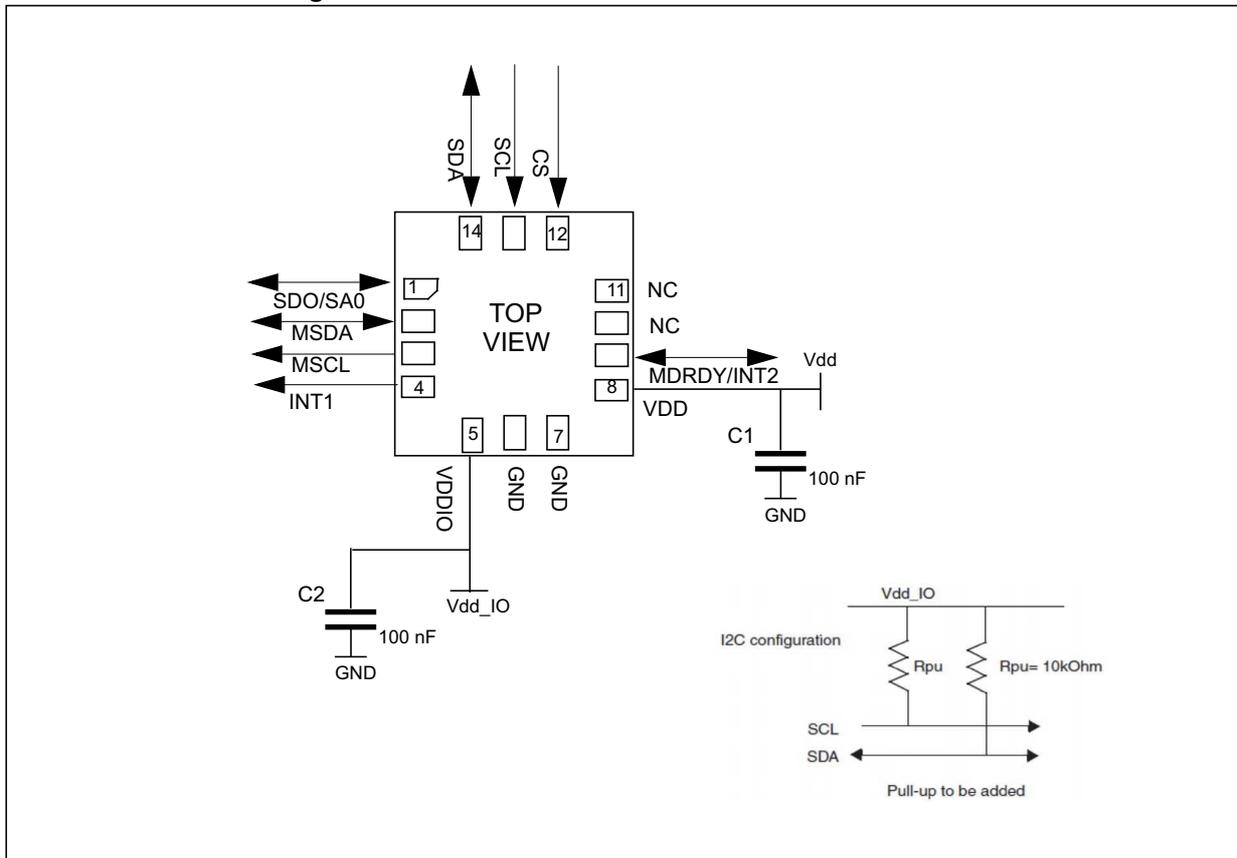
The device core is supplied through the Vdd line. Power supply decoupling capacitors (C1, C2 = 100 nF ceramic) should be placed as near as possible to the supply pin of the device (common design practice).
