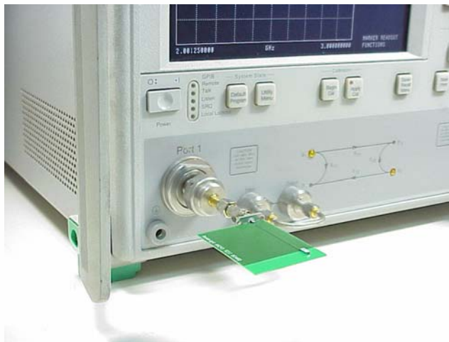
Testing Instrument: Anritsu 37369C VNA(Vector Network Analyzer)
