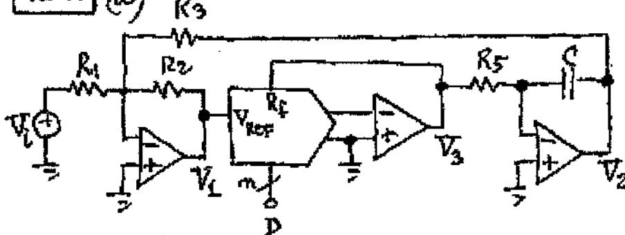
$$V_1 = -\frac{R_2}{R_1} V_i - \frac{R_2}{R_3} V_2; V_2 = -\frac{1}{sR_5C} V_3 = \frac{D}{sR_5C} V_1$$
