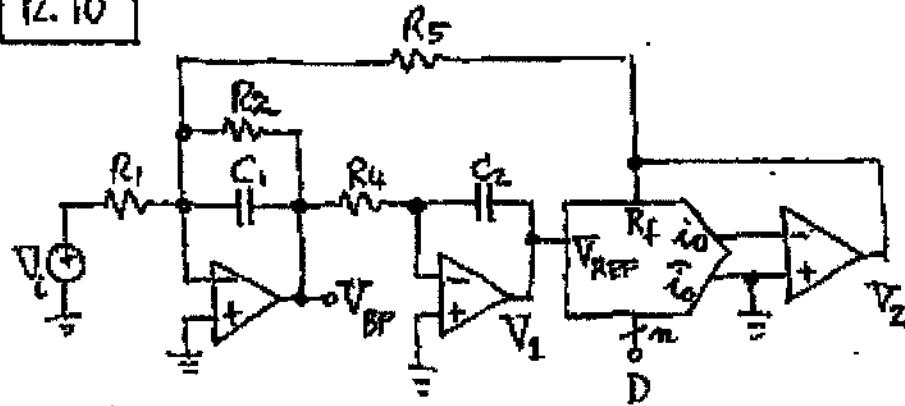
$$V_2 = -DV_1 = -\frac{-D}{5R_4C_2}V_{BP} = \frac{1}{5(R_4/D)C_2} \Rightarrow R_4 \rightarrow \frac{R_4}{D};$$
