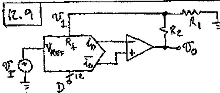
$$V_I = -DV_T; \quad \frac{0-V_I}{R_f} + \frac{0-V_I}{R_1} = \frac{V_I-V_O}{R_2}$$
