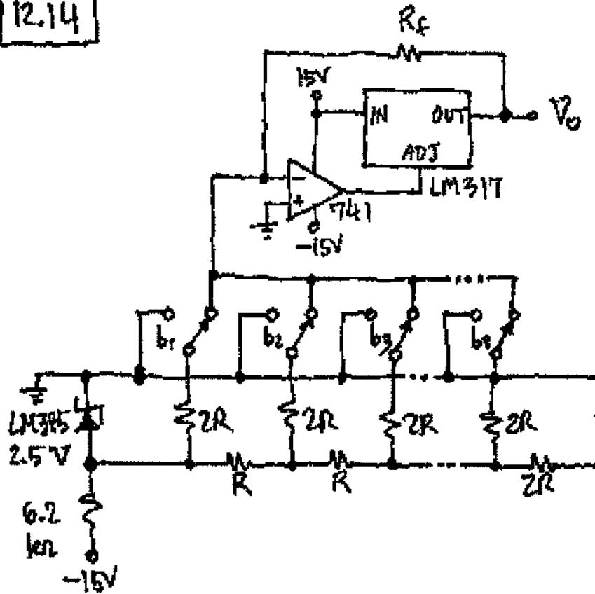
Use the LM 311 to boost the output current capability of the op amp. Assume  $R = 10\text{ k}\Omega$ , and use a  $6.2\text{ k}\Omega$  resistor to bias the reference diode and ladder. To find  $R_f$ , impose
