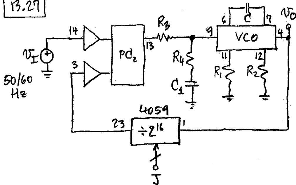
Design for  $f_I = 55 \text{ Hz}$ . Then,  $f_o = 55 \times 2^{16} = 3.60 \text{ MHz}$ . Arbitrarily impose  $2f_R = 2 \text{ MHz}$ , so that  $K_v = 2\pi \times 2 \times 10^6 / (3.9 - 1.1) = 4.49 \text{ (Mrad/s)}/\text{V}$ . To meet these specifications, the PLL Design Program suggests using  $R_1 = 22 \text{ k}\Omega$ ,  $R_2 = 39 \text{ k}\Omega$ , and  $C = 100 \text{ pF}$ .
