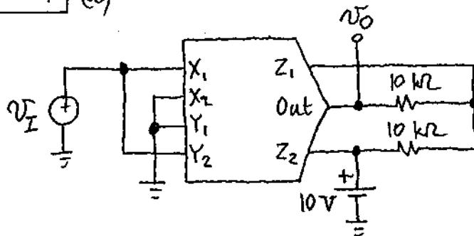
$$V_{Z_1} = \frac{1}{2}(V_O + 10 \text{ V}); \quad V_{Z_2} = 10 \text{ V}; \quad V_{Z_1} - V_{Z_2} = \frac{1}{2}V_O - 5 \text{ V}.$$
