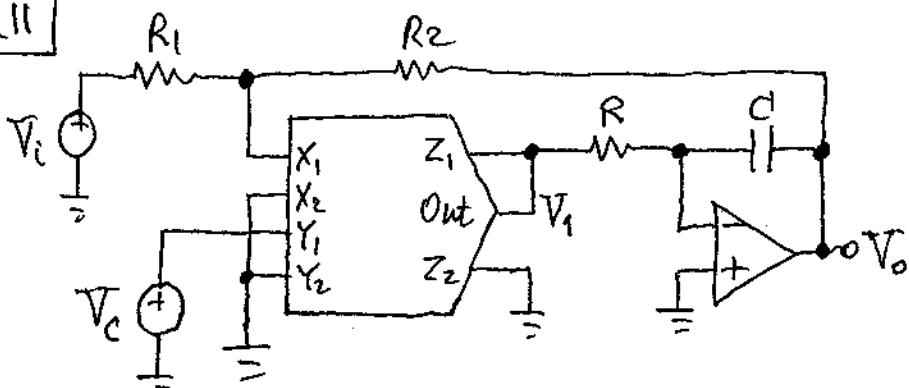
$$V_0 = -[1/(SRC)]V_1, \quad V_1 = \left( \frac{R_2}{R_1+R_2} V_i + \frac{R_1}{R_1+R_2} V_o \right) \frac{V_d}{10}.$$
