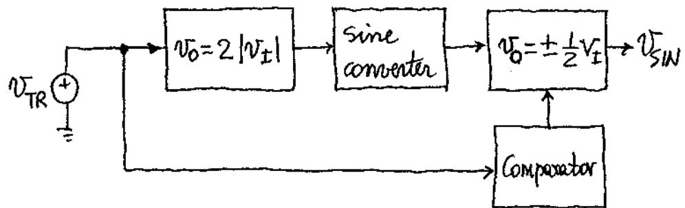
For the absolute-value circuit use Fig. (9.30) with  $R_1 = R_2 = 2R_3 = R_4 = R_5/2 = 10.0 \text{ k}\Omega$ . For the sine converter use part (a) above. For the polarity detector and programmable gain amplifier use the accompanying circuit.
