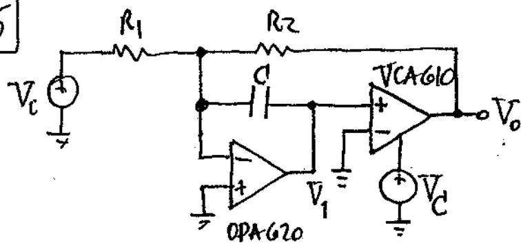
$$V_1 = -\frac{1}{SR_1C}V_i - \frac{1}{SR_2C}V_o; \quad V_o = 0.01 \times 10^{-2}V_d \times V_1.$$
