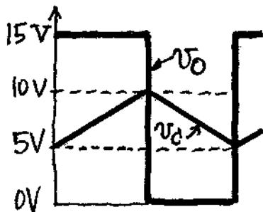
OTA inputs are  $V_P = 2.5 \text{ V}$  and  $V_N = 1.36 \text{ V} \Rightarrow \text{OTA's input stage saturates such that OTA sources}$
