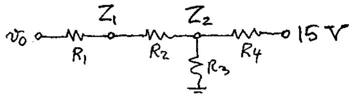
We want  $V_{Z_1} - V_{Z_2} = \frac{1}{2}V_O - 5 \text{ V}$ . The Thévenin equivalent of the circuit to the right of  $R_2$  is a source  $15 R_3 / (R_3 + R_4)$  with a series resistance  $R_3 || R_4$ , so
