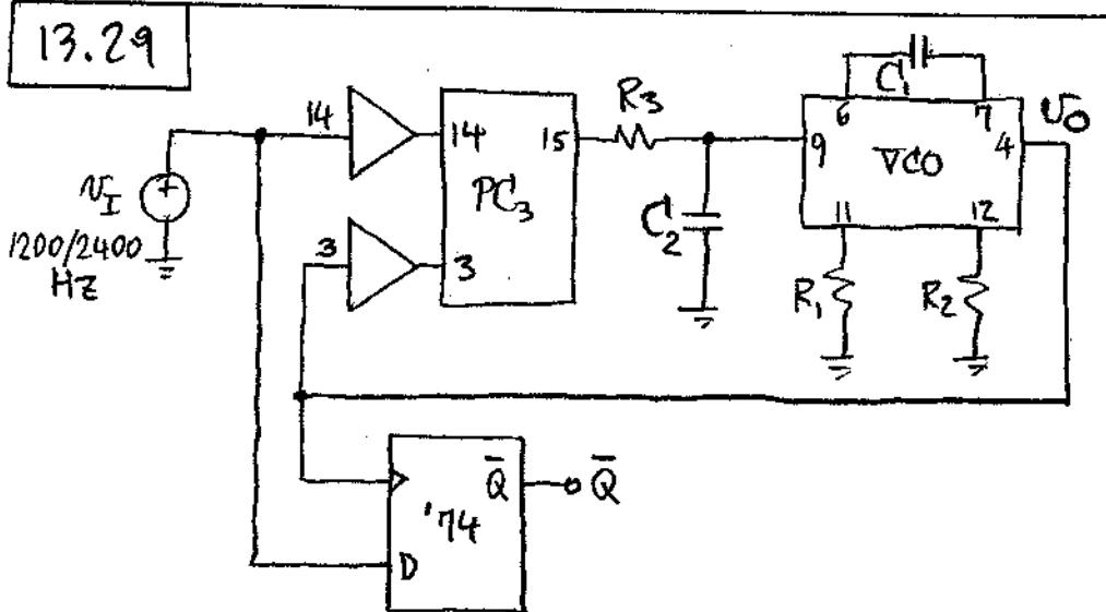
PLL Design program  $\Rightarrow C_1 = 33 \text{ mF}$ ,  $R_1 = 91 \text{ k}\Omega$ ,  $R_2 = 1.3 \text{ M}\Omega$ .  $R_3 C_2 = 1/2\pi f_H \Rightarrow C_2 = 33 \text{ mF}$ ,  $R_3 = 2 \text{ k}\Omega$ .
