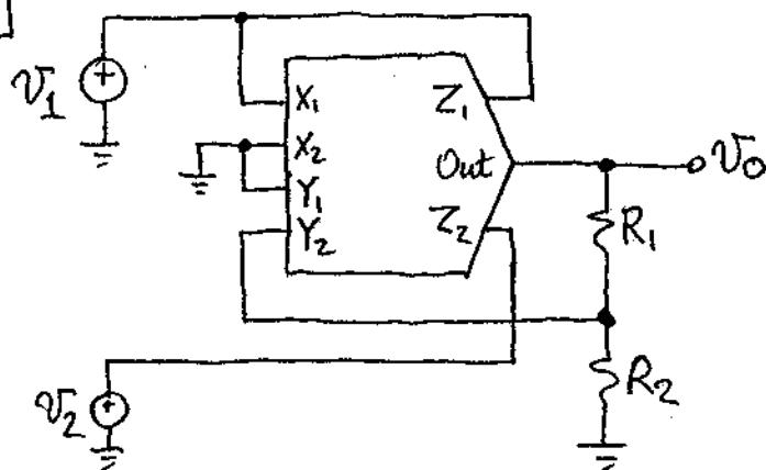
$$V_1 - V_2 = \frac{1}{10} (V_1 - 0) \times \left( 0 - \frac{R_2}{R_1 + R_2} V_O \right) \Rightarrow V_O = \left( 1 + \frac{R_1}{R_2} \right) 10 \frac{V_2 - V_1}{V_1}$$
