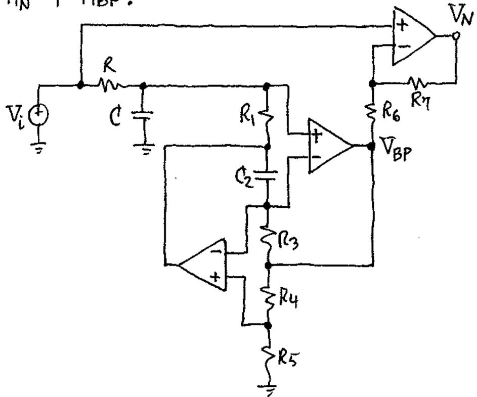
Let  $R_4 = R_5$ , so that  $V_{BP} = 2H_{BP}V_i$ ; let  $R_6 = R_7$ , so that  $V_N = 2V_i - 2H_{BP}V_i = H_{ON}H_NV_i$ ,  $H_{ON} = 2 V/V$ .
