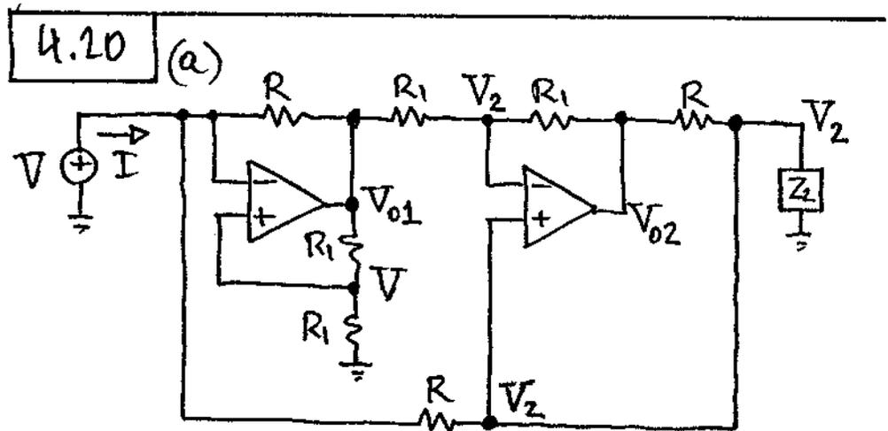
$$V_{o1} = 2V; \quad V_{o2} = -V_{o1} + 2V_2; \quad I = \frac{V - V_{o1}}{R} + \frac{V - V_2}{R}; \quad \frac{V - V_2}{R} = \frac{V_2 - V_{o2}}{R} + \frac{V_2}{Z_2} \cdot \text{Eliminating } V_{o1}, V_{o2}, \text{ and } V_2 \text{ and collecting, } Z_1 = \frac{V}{I} = \frac{R^2}{Z_2}$$
