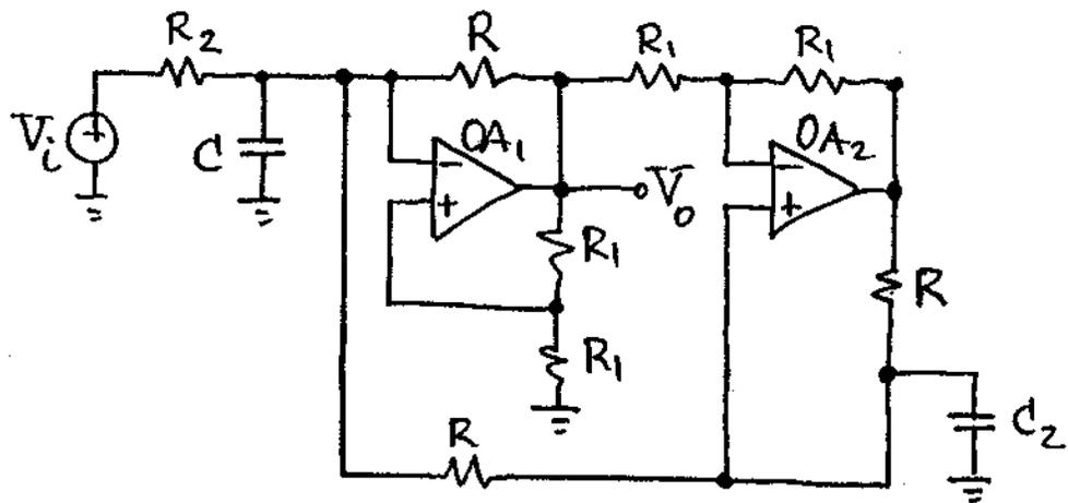
Let  $C = 1 \mu\text{F}$ . Then,  $L = 1/[(2\pi f_0)^2 C] = 1/[(2\pi)^2 10^{-6}] = 25.33 \text{ KH}$ . Use  $C_2 = 1 \mu\text{F}$ ,  $R = \sqrt{L/C_2} = \sqrt{25,330 \times 10^6} = 158 \text{ k}\Omega$ ,  $R_1 = 100 \text{ k}\Omega$ ,  $R_2 = Q \sqrt{L/C} = 10 \sqrt{25,330 \times 10^6} = 1.58 \text{ M}\Omega$ . Obtain  $V_0$  from  $OA_1$ 's output, where the output impedance is low. Then,  $H_{\text{OBP}} = 2V/V$ .
