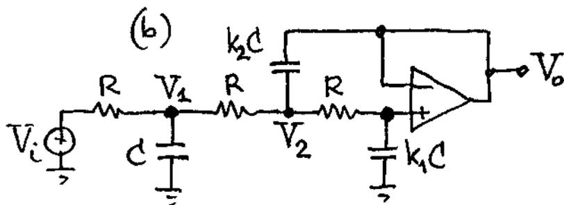
$$V_o = \frac{1}{1 + j\omega k_1 RC} V_2 \Rightarrow V_2 = (1 + j\omega k_1 RC) V_o.$$
