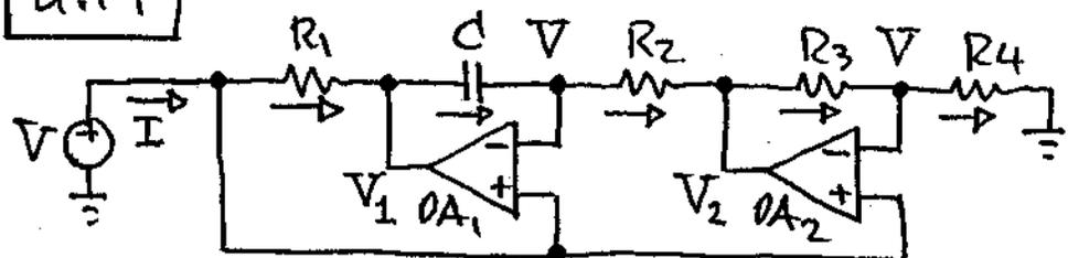
$$I = \frac{V - V_1}{R_1}; \quad j\omega C(V_1 - V) = \frac{V - V_2}{R_2}; \quad V_2 = \left(1 + \frac{R_3}{R_4}\right) \times V.$$
