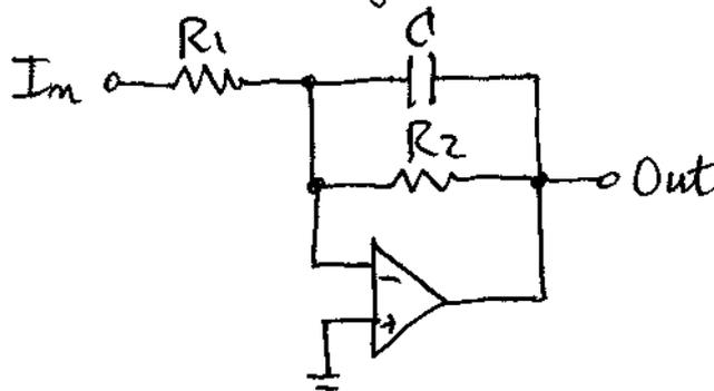
$$\text{with } \omega_0 = \frac{1}{R_2 C} \quad H_0 = -\frac{R_2}{R_1}.$$
