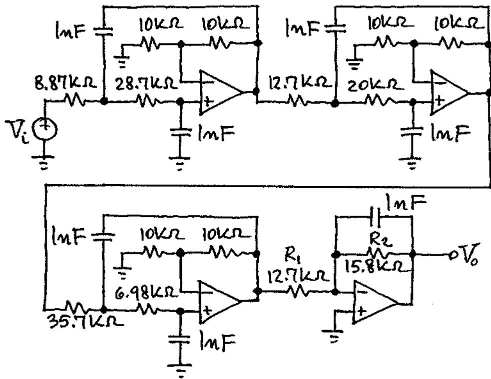
4.11 From Table 4.1 we see that we need two second-order stages with  $f_{01} = 360/0.994 = 362.17\text{Hz}$ ,  $Q_1 = 5.556$ , and  $f_{02} = 360/0.655 = 549.62\text{Hz}$ ,  $Q_2 = 1.399$ ; and a first-order stage with  $f_{03} = 360/0.289 = 1,245.7\text{Hz}$ .
