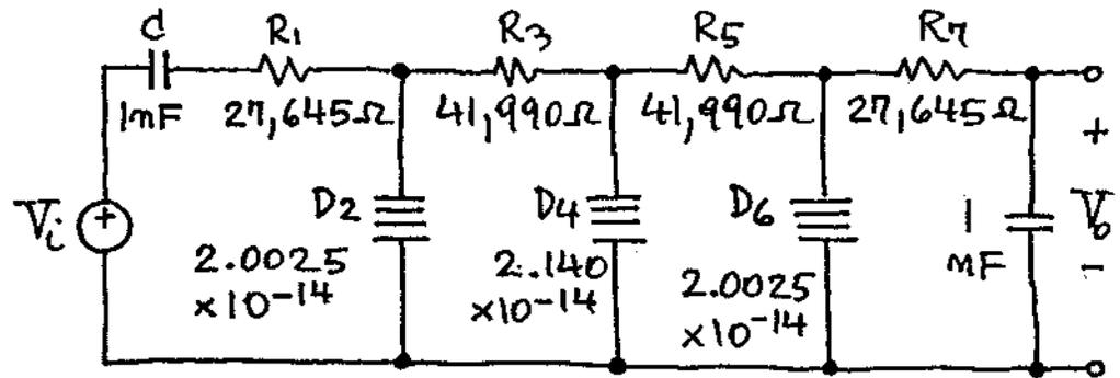
In the FDNRs let  $C_1 = C_3 = 1\text{mF}$ ,  $R_2 = R_5 = R_4$ . Then,  $D = R_2 C_1^2 \Rightarrow R_2 = D/C_1^2 = 10^{18} D$ . Thus, for  $D_2$  and  $D_6$  we have  $R_2 = R_5 = R_4 = 10^{18} \times 2.0025 \times 10^{-14} = 20.025 \text{ k}\Omega$ . For  $D_4$  we have  $R_2 = R_5 = R_4 = 10^{18} \times 2.140 \times 10^{-14} = 21.4 \text{ k}\Omega$ .
