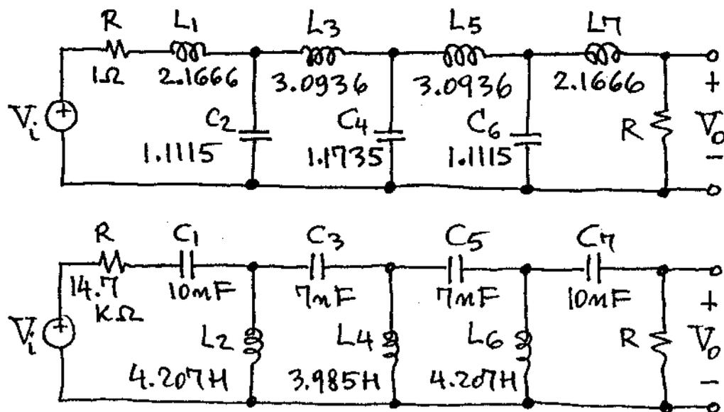
To find the element values in the GICs, impose equal resistances and  $C = 10$  mF throughout. For the 1st and 3rd GIC we obtain  $R_k^2 = 4.207 / 10^{-8} \Rightarrow R_k = 20.51$  K $\Omega$ . For the 2nd GIC,  $R_k^2 = 3.985 / 10^{-8} \Rightarrow R_k = 19.96$  K $\Omega$ . Actual implementation:
